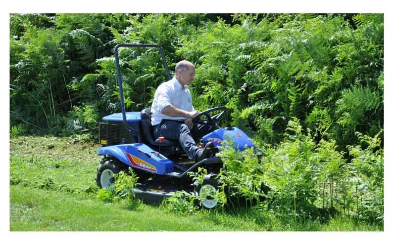
The SRA800 and SRA950F are ride-on brush cutters capable of cutting grass and thick vegetation right up to saplings. Their low height aids stability when used on slopes.
