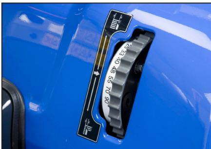
"Dial-in" cutting height adjustment
