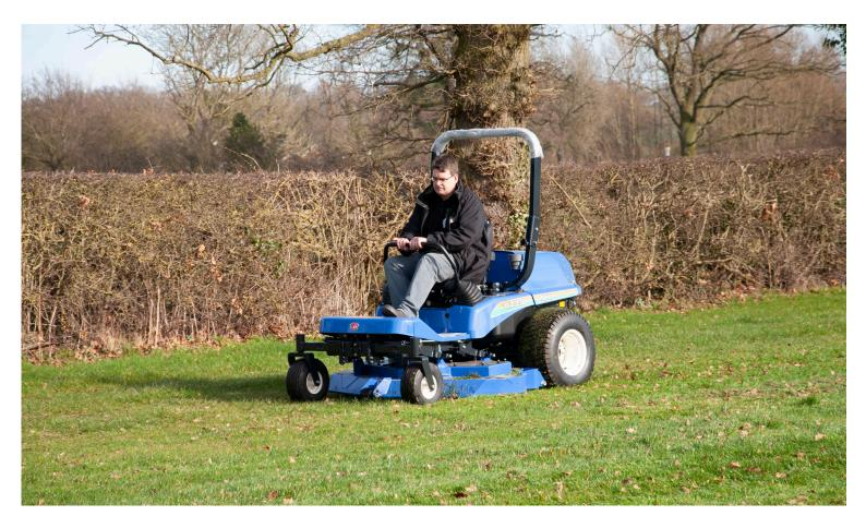
A zero turn mower, the ISEKI SZ330 is offered with a choice of 1.6m or 1.8m rear cutting decks. Powered by a 33hp three-cylinder, liquid cooled diesel engine, which is easily accessed via the tilting one-piece engine cover. A mulching kit is available for the rear discharge decks.
