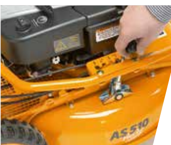
CENTRAL HEIGHT ADJUSTMENT Spring supported, central height adjustment (40 – 90 mm or 30 – 80 mm).
