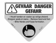
This sticker is attached to the safety net and warns against the danger of injury to hands. The screen on the shredding chamber should only be opened once the knives have come to a complete standstill. The motor should always be switched off before lifting the safety net.
