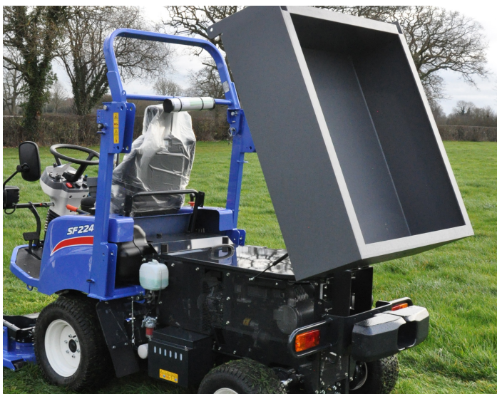
Storage box tips for easy service access.
