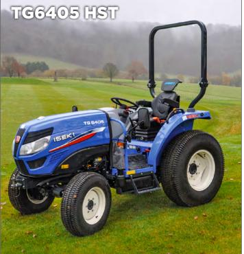
The TG6045 HST features the new 2-stage servo hydrostat transmission offering 3 three speeds with high and low ranges. TG6405 has a three speed HST. Both tractors have an electronic shuttle lever plus controls for maximum speed, hydrostat response and cruise control with resume speed memory function.
