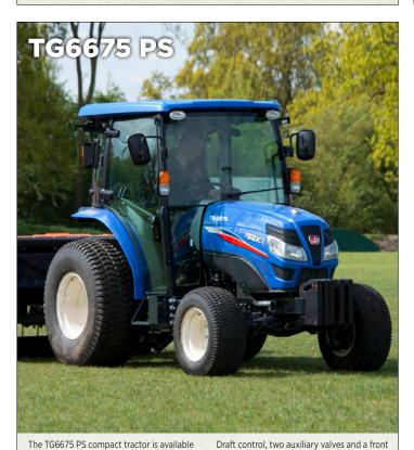
with a ROPS or a factory fitted, fully air-conditioned category 2 cabin. It features a 65hp four cylinder, Stage IIIB diesel engine, with a F12/R12 power-shuttle transmission. The rear, category 1 & 2, 3-point linkage has a capacity of 1,600kg at ball end and 1,500kg at 24 inches.
