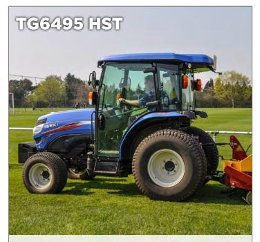
The TG6495 HST features the 2-stage servo hydrostat transmission offering three speeds with high and low ranges. It has an electronic shuttle lever plus controls for maximum speed, hydrostat response and cruise control with a resume speed memory function.
