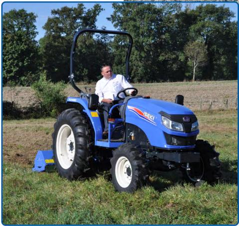
Perfect for multi-users the easy to operate tractor is available in two models, the 38hp TLE3400 with hydrostatic transmission or the 47hp TLE4490 with mechanical transmission for the ultimate control.
