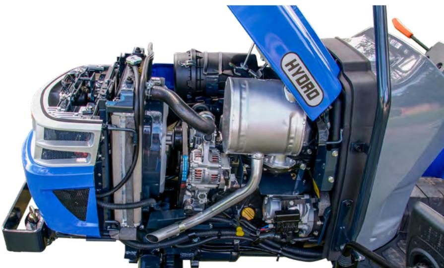
Powered by a reliable high capacity 1,123cc or 1,498cc three-cylinder diesel, water cooled engine. Available with Stage V Compliant 19hp or 25hp engines which offer efficient operation at low 2,600rpm for decreased noise levels, improved operator comfort and less wear on the engine.
